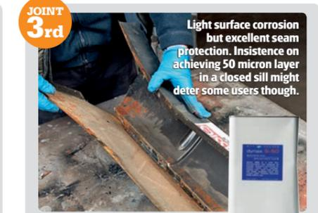
**JOINT 3rd** Light surface corrosion but excellent seam protection. Insistence on achieving 50 micron layer in a closed sill might deter some users though.
