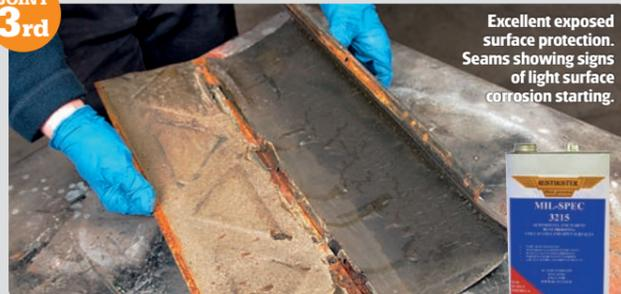
Excellent exposed surface protection. Seams showing signs of light surface corrosion starting.
