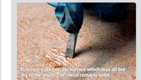
Fine rust tracks on the surface which was all but dry to the touch. The metal remains solid.
