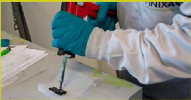
**06 PRESS THE PRODUCT FROM THE INSIDE OUT TO THE AESTHETIC SIDE OF THE REPAIR SPOT THRU THE HOLES.**
