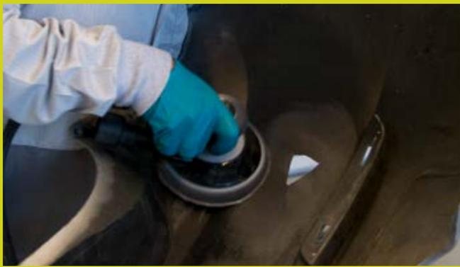
**03 PIN HOLES ALONG EACH SIDE OF THE REPAIR in the V groove area**
