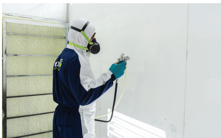
CPP 17 being applied via spray gun.
