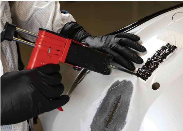
Plastic repair in application.
